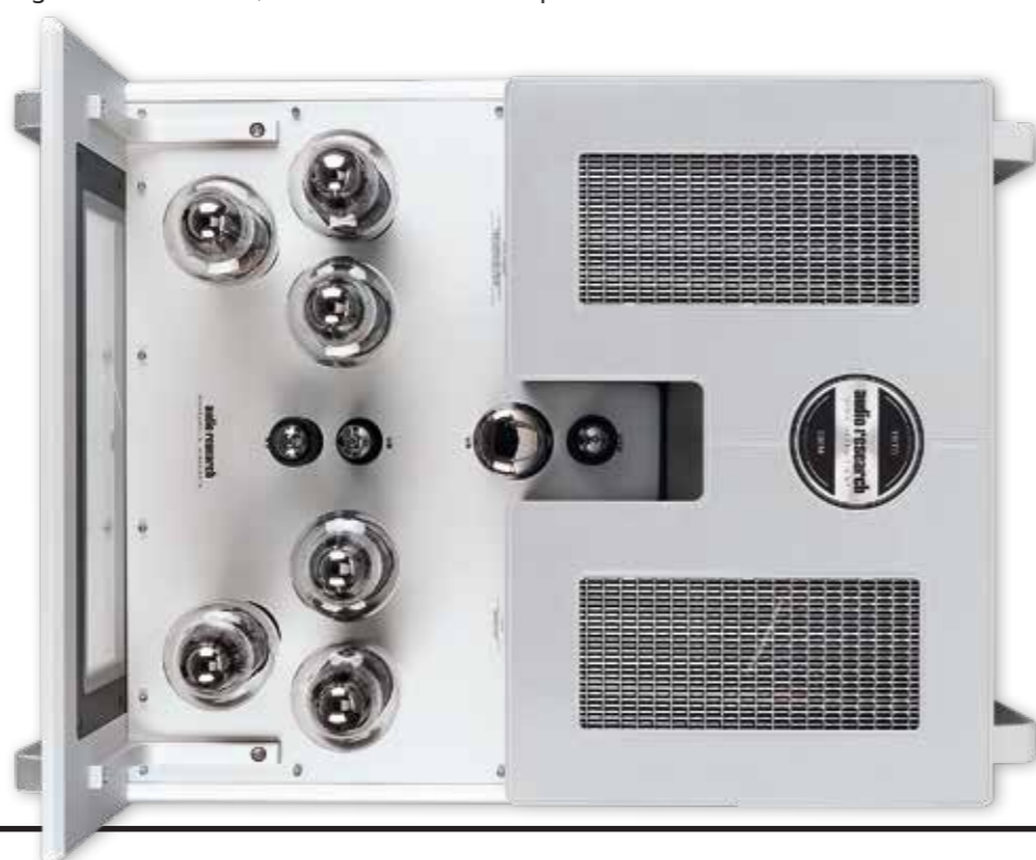
RIGHT: The three pairs of KT170 output tubes [see boxout p44] are revealed alongside the ECC83/6H30 input/voltage gain triodes (and 6H30/6550 for PSU regulation). The PSU and output transformers are screened at the rear
